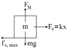
$$F_e = f_{s,max} \xrightarrow{f_{s,max} = \mu_s F_N} kx = \mu_s mg$$
