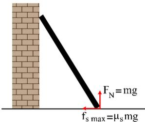
$$R_{max} = \sqrt{F_N^2 + f_{s \text{ max}}^2} = \sqrt{(mg)^2 + (\mu_s mg)^2} = mg \sqrt{1 + \mu_s^2}$$
