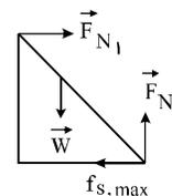
$$f_{s,max} = F_{N1} = \mu_s F_{N2} \xrightarrow[\mu_s = 0,5]{F_{N2} = W} f_{s,max} = F_{N1} = 0,5W$$
