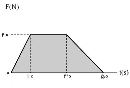
$$S = \Delta p \xrightarrow{\Delta p = F_{netav} \cdot \Delta t} F_{netav} = \frac{\Delta p}{\Delta t} = \frac{S_{F-t}}{\Delta t} \Rightarrow F_{netav} = \frac{50+20}{2} \times 20 \Rightarrow F_{netav} = 14N$$
